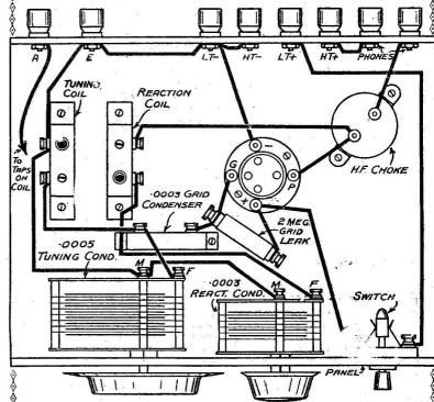
the pin side of the reaction-coil holder. Wire-up with thick insulated wire, removing the insulation where wires hook under terminals.
