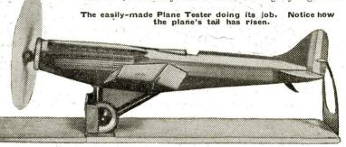
THIS plane tester is not able to show up every fault in a model aeroplane, of course, so after putting your model through its paces on the tester you should give it a few trial flights.
